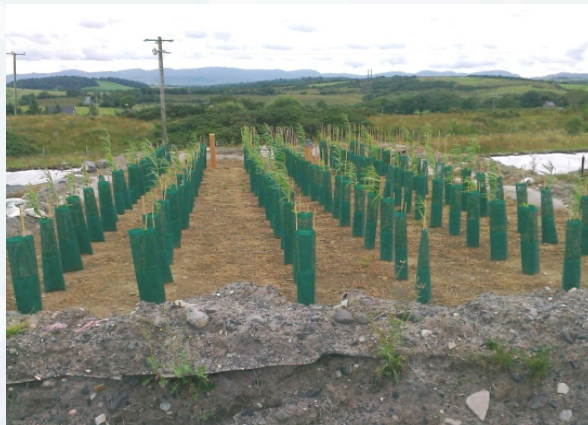
Ballynacarrick Landfill site 12 Lysimeters irrigated under 4 irrigation regimes
