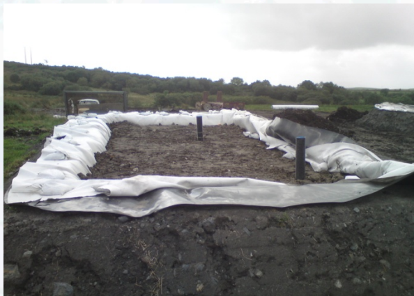
Ballynacarrick Landfill site 12 Lysimeters irrigated under 4 irrigation regimes
