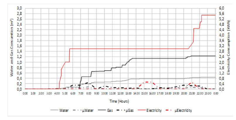
example of the type of results that can be obtained through the instrumentation and monitoring of household consumption
