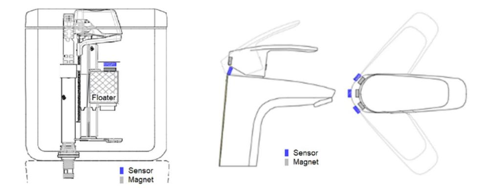
Placement of sensors on taps and toilet flush
