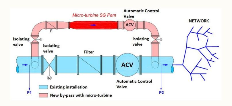
Easy and common assembly: in parallel with the already applied pressure reducing valves
