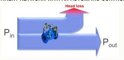
Head loss (Pin – Pout) by cavitation Reduces service life of the automatic control valve
