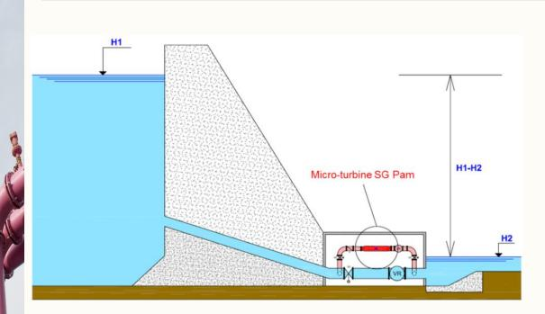
Ecological compulsory flows in Dams: in the chamber of the flow regulating valve
