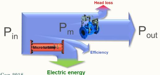
Reducing Head loss = (P<sub>in</sub> – Pout) = increase service life of the ACV
